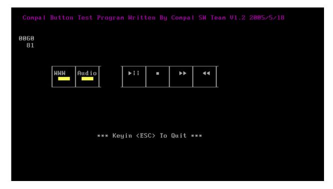
Press each of the buttons on the front panel in turn. A yellow bar will appear on the relevant section of the figure if the button passes the test.
