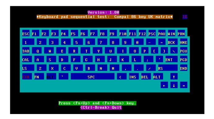
Pressing a key also reveals that key's **scan codes** in the upper right hand corner of the screen. When the key is depressed, its **make code** is displayed. When the key is released, the **break code** is shown.
